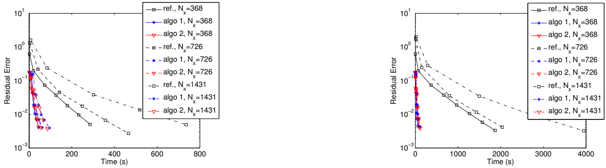
Figure 28: Influence of the dimension of approximation spaces. Residual error versus computation time for the reference solver and GSD algorithms 1 and 2 for different N_x and for N_o = 4 (left plot) or N_o = 5 (right plot)
