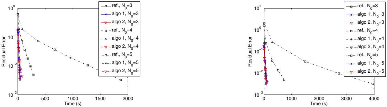
Figure 29: Influence of the dimension of approximation spaces. Residual error versus computation time for the reference solver and GSD algorithms 1 and 2 for different N_o and for N_x = 368 (left plot) or N_x = 1431 (right plot)
