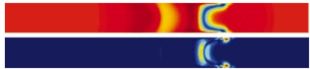
FIG. 11. (Color) Mean (top) and standard deviation (bottom) of the electrical conductivity of the electrolyte solution at t = 0.50 s. Annihilation of ions in the labeling reaction results in a significantly lower mean electrical conductivity near the L plug. The values of the contour levels go linearly from 7.1 \times 10^{-3} S/m (blue) to 1.3 \times 10^{-2} S/m (red) in the top plot and from 0 (blue) to 1.5 \times 10^{-3} S/m (red) in the bottom plot.
