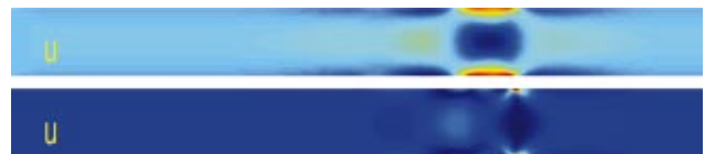
FIG. 14. (Color) Mean (top) and standard deviation (bottom) of the streamwise velocity at t = 0.50 s. The local increase in the electroosmotic wall velocity leads to recirculation zones near the L plug. The largest uncertainties are found near the wall. The values of the contour levels go linearly from 6.8 mm/s (blue) to 9.1 mm/s (red) in the top plot and from 5.6 \times 10^{-3} mm/s (blue) to 0.59 mm/s (red) in the bottom plot.
