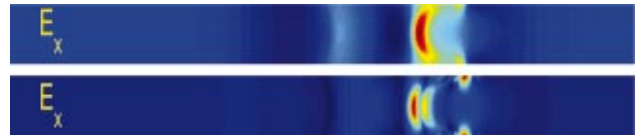
FIG. 12. (Color) Mean (top) and standard deviation (bottom) of the electrical field strength in the x direction at t = 0.50 s. Near the L plug, the mean streamwise electrical field strength is about 40% higher than in the undisturbed flow. The values of the contour levels go linearly from 91.4 kV/m (blue) to 146 kV/m (red) in the top plot and from 0.20 kV/m (blue) to 13 kV/m (red) in the bottom plot.
