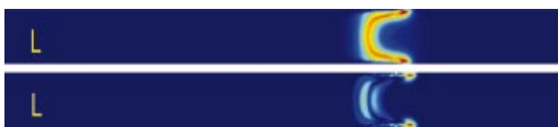
FIG. 10. (Color) Mean (top) and standard deviation (bottom) of the labeled protein concentration L at t = 0.50 s. The initially flat profiles are now severely distorted. The values of the contour levels go linearly from 0 (blue) to 3.2 \times 10^{-4} mol/l (red) in the top plot and from 0 (blue) to 10^{-4} mol/l (red) in the bottom plot.
