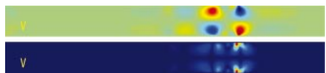
FIG. 15. (Color) Mean (top) and standard deviation (bottom) of the wall-normal velocity at t = 0.50 s. The mean of this velocity has a magnitude of up to 6% of the initial streamwise velocity. The values of the contour levels go linearly from -0.56 mm/s (blue) to 0.56 mm/s (red) in the top plot and from 0 (blue) to 0.26 mm/s (red) in the bottom plot.
