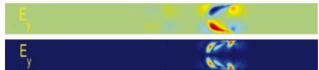
FIG. 13. (Color) Mean (top) and standard deviation (bottom) of the electrical field strength in the y direction at t = 0.50 s. The magnitude of the mean of this field strength is up to 15% of the initial field strength in the x direction. The values of the contour levels go linearly from -16.3 kV/m (blue) to 16.3 kV/m (red) in the top plot and from 0 (blue) to 5.8 kV/m (red) in the bottom plot.
